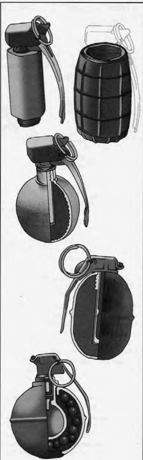
Top to Bottom: Diehl HGR DM51 (offensive), Diehl HGR DM51 (defensive fragmentation sleeve), SM HG 85 (sectioned), Bazalt RGN-86 (sectioned), and Precision Ordnance M452 stingball (sectioned).
